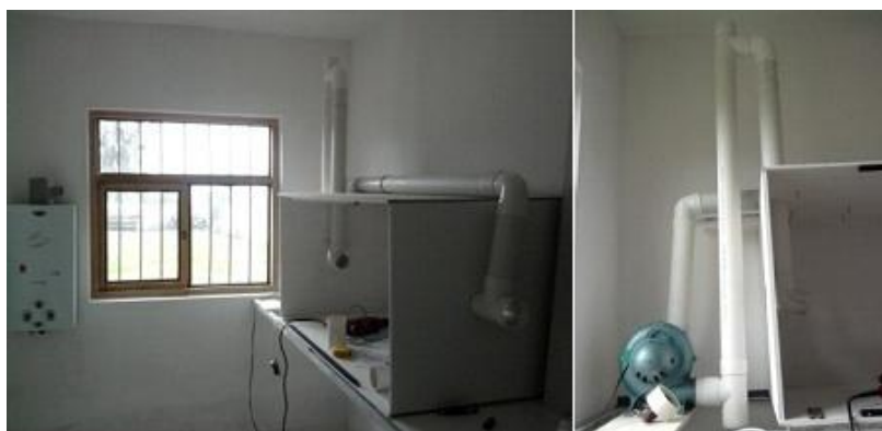
Figure 2. Experimental bioreactor built at the CEBA for the SSF by Pleurotus
