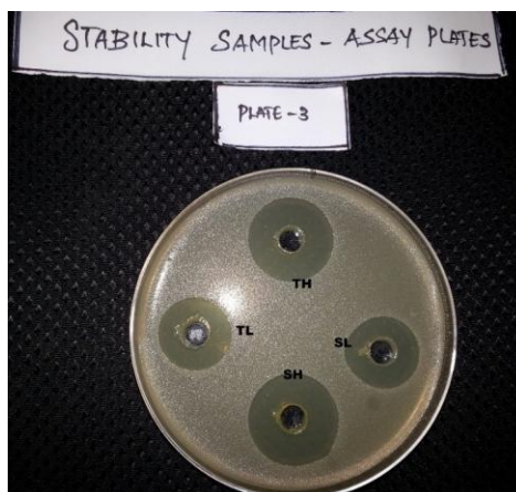
FIG-24: Stability samples –Assay Plate No: 3(TH-Test High, TL-Test low, SH- Standard High, SL- Standard low)
