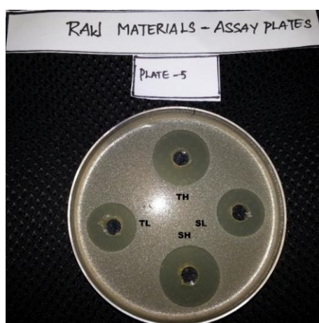
FIG-11: Raw Materials – Assay Plate No:5(TH-Test High, TL-Test low, SH- Standard High, SL-Standard low)
