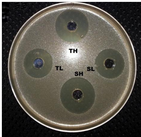
FIG-13: Validation Samples - Assay Plate No: 2 (TH-Test High, TL-Test low, SH- Standard High, SL- Standard low)
