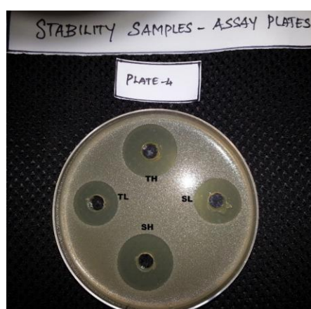
FIG-25: Stability samples –Assay Plate No: 4 (TH-Test High, TL-Test low, SH- Standard High, SL- Standard low)
