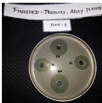
FIG-17: Finished Products– Assay Plate No: 1(TH-Test High, TL-Test low, SH- Standard High, SL- Standard low)
