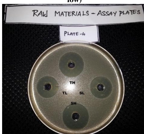
FIG-10: Raw Materials – Assay Plate No: 4(TH-Test High, TL-Test low, SH- Standard High, SL-Standard low)
