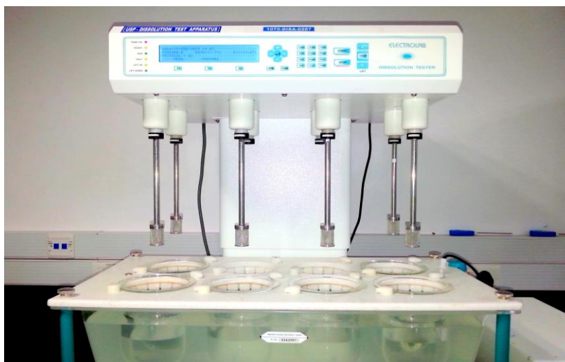
Fig- 4 Shows the digitalized dissolution apparatus.
