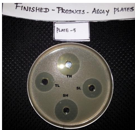
FIG-21: Finished Products –Assay Plate No: 5 (TH-Test High, TL-Test low, SH- Standard High, SL- Standard low)
