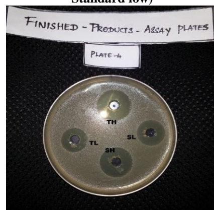
FIG-20:Finished Products– Assay Plate No: 4(TH-Test High, TL-Test low, SH- Standard High, SL- Standard low)
