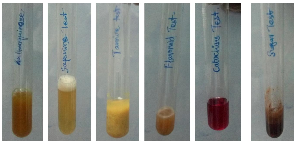
Figure 3: Phytochemical analysis of A. latifolia (Roxb.) 5g plant powder was weighed in butter paper and extracts of different solvents, ranging from water to n-hexane (in order of polarity), were prepared. Qualitative phytochemical analysis was carried out as per the method of Brindha et al. From left to right: Catechins, sugars, tannins, anthraquinones, flavonoids and saponin tests.
