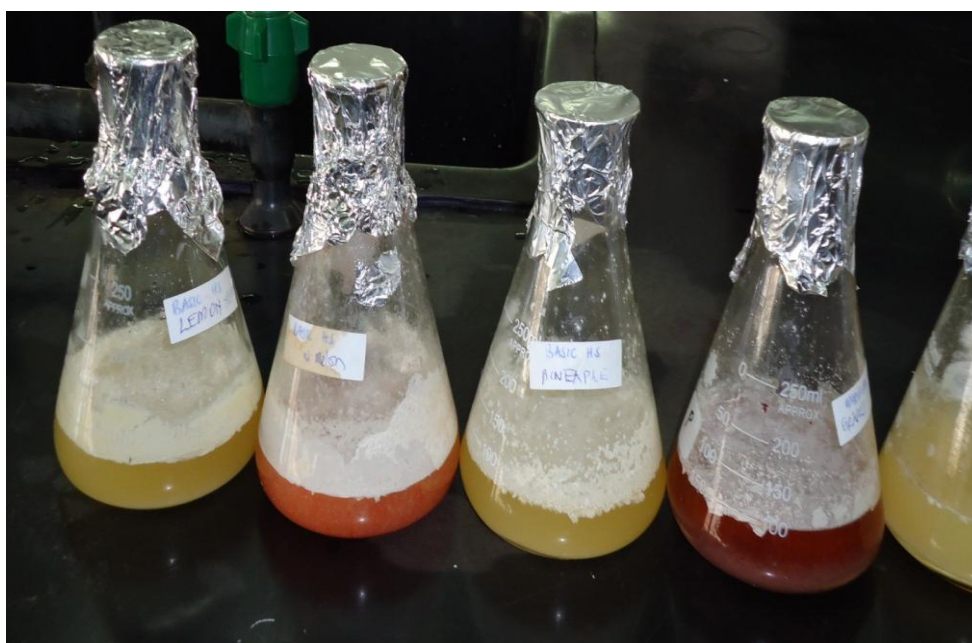
Fig. 7: On the fourth day the flasks were covered with a thick pellicle to signify for presence of cellulose synthesizing bacteria.
