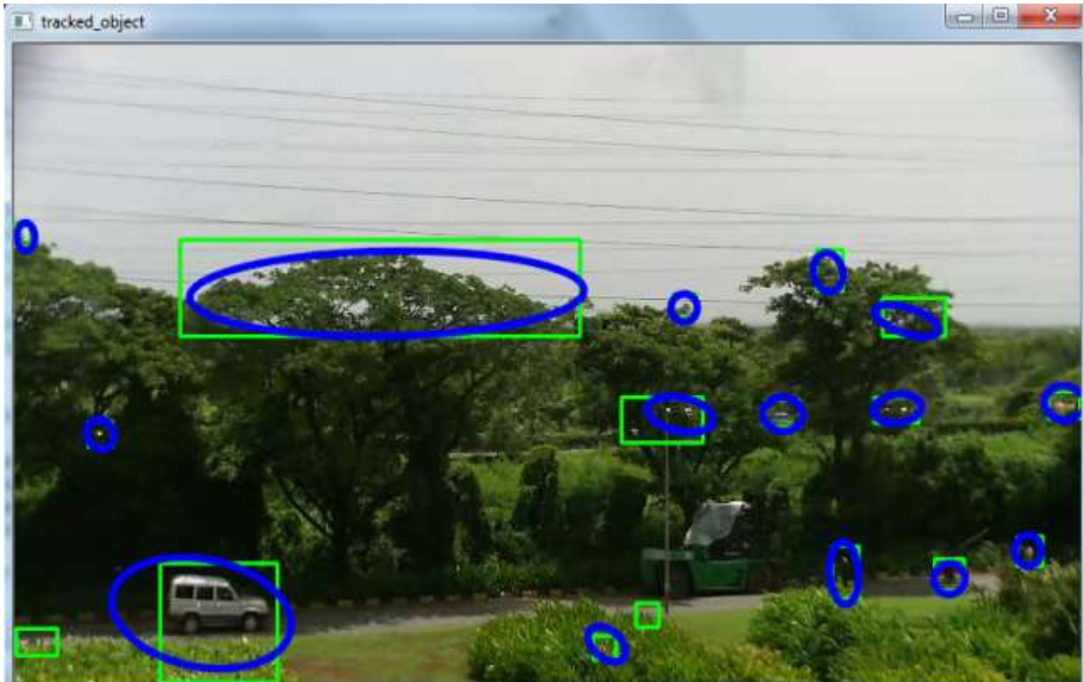
Fig 5. After calling CAMshift Algorithm, Ellipse is getting drawn around only those motion contours which are getting tracked in consecutive frames.
