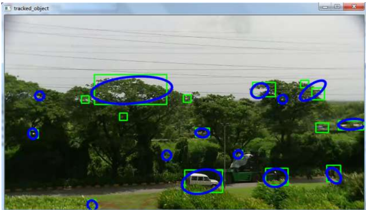
Fig 6. After calling CAMshift Algorithm, Ellipse is getting drawn around only those motion contours which are getting tracked in consecutive frames.
