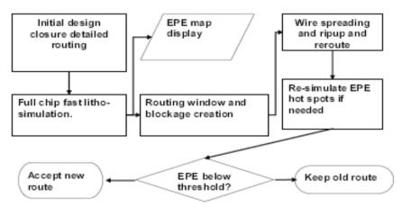
Fig. 1. EPE based construct-by-correction in the model-based method [4].
