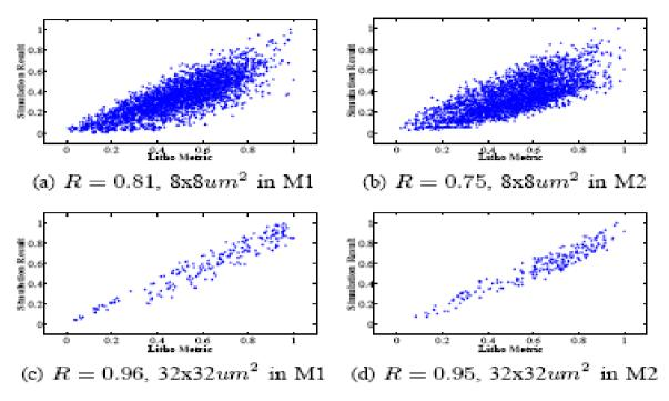
Fig. 3. The litho-metric shows higher fidelity to post-OPC printability in large scale.
