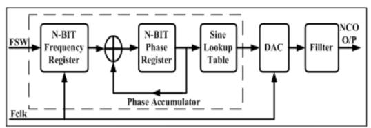
Fig 1. Block Diagram of a NCO system
