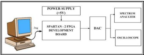
Fig.7 Block Diagram of Experimental Setup
