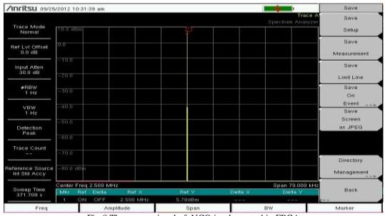
Fig.8 The output signal of NCO implemented in FPGA
