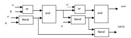
Figure 6: Proposed NAND, AND & OR gate full adder architecture
