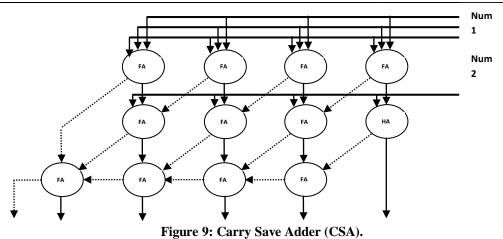
The multi bit binary addition is the most important operation used in arithmetic operation on digital video / image processors. Hence multi bit adders are the most important blocks in building digital systems. The key challenge addressed in this work is the low power multi bit adders.
