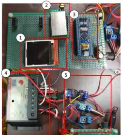
1-Display monitor; 2-LoRa Module; 3-Microcontroller STM32F103C8T6; 4-Solar charger DC/DC; 5-Voltage and current sensors
