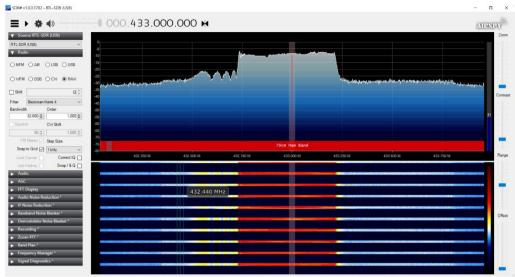
**Figure4.** Spectrum analysis of LoRa signal transmited from E32-TTL-100 module with default parameters (2400bps)
