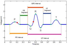
Fig.2: Main characteristics of an ECG curve
