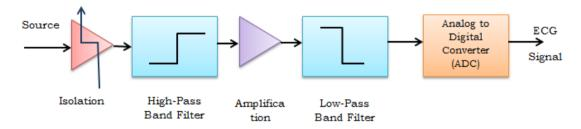
Fig.1: Architecture for acquisition of an ECG
