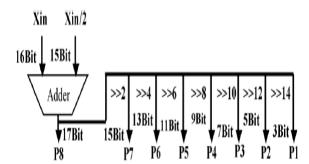
Fig3: Block diagram of the Partial Product Generator Unit.
