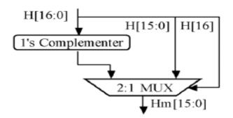
Fig2: Hardware architecture of the Sign Conversion Block.
