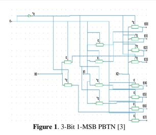
After 3-bit PBTN is established, 4-bit PBTN can be built by connecting two of 3 bit 1-MSB PBTN. The first 3 bits of binary code input was connected to 2 blocks of 3-bit 1-MSB PBTN. LSB X0 of the input bit was connected to 2 extra transmission gates, and its output was connected to output line t3 and t7 as shown in Figure 2. The 10-bit 1-MSB PBTN can be built after 9-bit PBTN is established.
