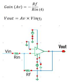
Figure 4. Configuration of Inverting Amplifier
