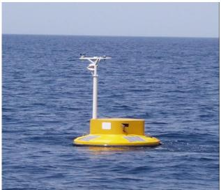
Fig 2: Ambient Noise Buoy
