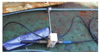
Fig 1: Hydrophone with fixture
