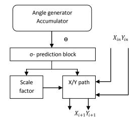
Fig 2 Block schematic of the proposed system
