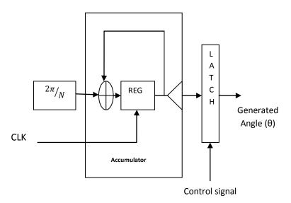
Fig 3  $\theta$ - generator of the proposed system.
