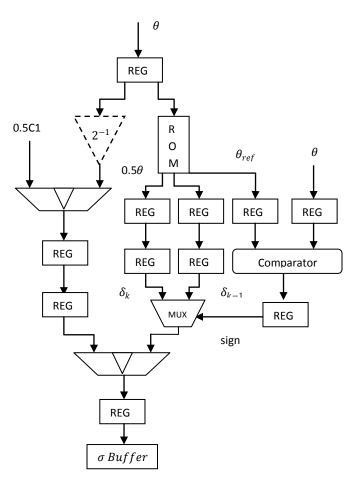
Fig.5 Realization of direction of rotation for an angle using  $\sigma$  –prediction
