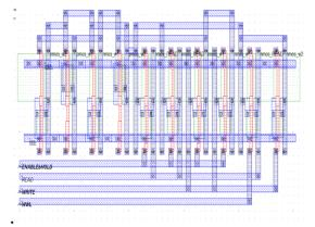
Figure 5: Layout Design of 8T-SRAM
