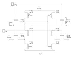
Figure 2: ST1 Bit Cell
