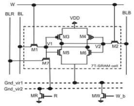
Figure 3: Virtual Grounding Based Read Error Reduced SRAM Cell
