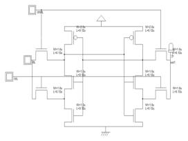
Figure 1: ST2 Bit Cell
