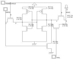
Figure 4: Read Error Reduced 8T-SRAM Cell with Reduced Transistor Count
