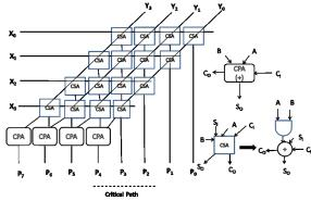
Fig 5.6 Architecture of 4 bit multiplier
