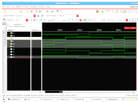
Fig 13 Output waveform of Reversible D latch with Control signals using Toffoli gate
