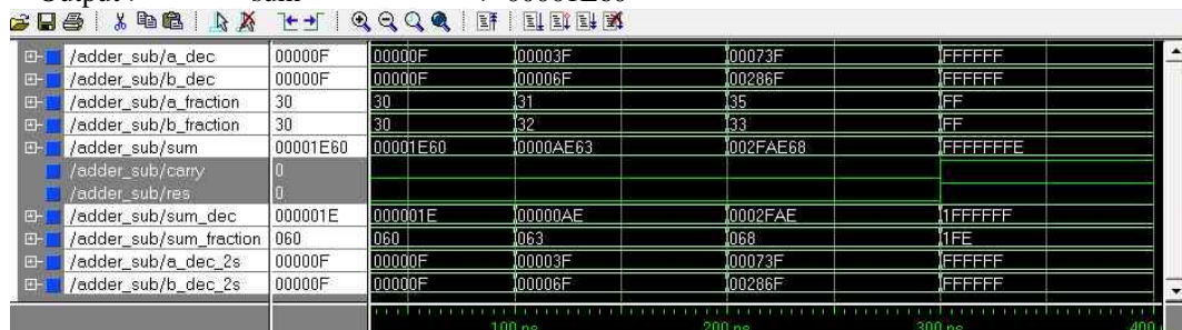
Figure 6: Simulation Waveform of Fixed Point Add/Subtract Code
