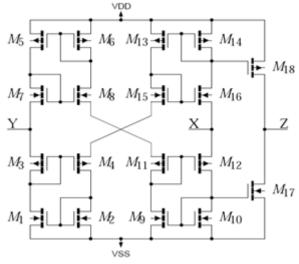
Fig. 1.Schematic of CCIII
