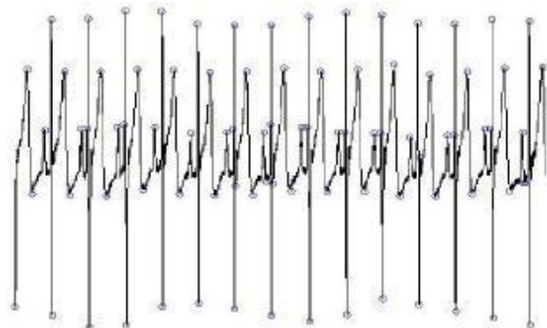
Figure 7: Detected positive and negative R-waves in FECG signal according to proposed algorithm
