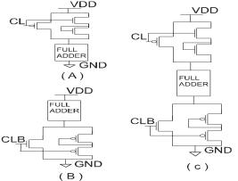
Fig.4 Full Adder with (A) USVL (B) LSVL (C) SVL technique
