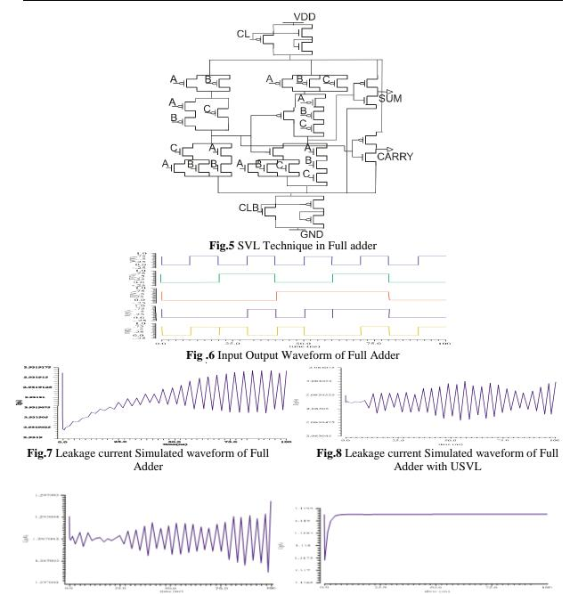
Fig.9 Leakage current Simulated waveform of Full Adder with LSVL technique
