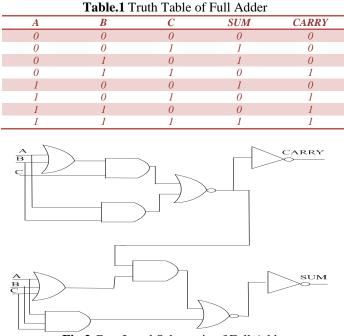
**Fig.2** Gate Level Schematic of Full Adder
