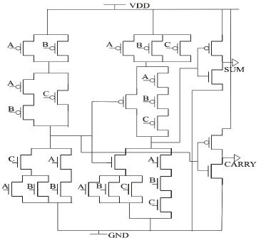
Fig.3 Transistor level schematic of Full Adder
