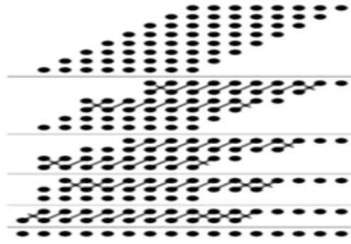
Fig 4: Method of Reduction on 8x8 Multiplier.
