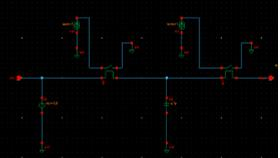
Fig 2. Switched Capacitor circuit
