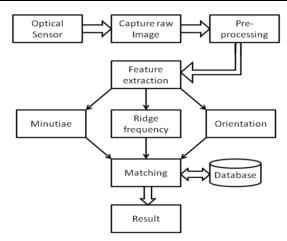
Fig No. 1 Block diagram for implemented FKP Authentication using minutiae.
