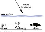
Fig.2 Underwater image acquisition
