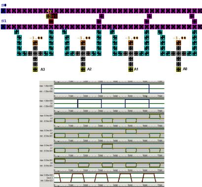
Fig. 13 Layout and Simulation Result of QCA based 2:4 decoder circuit using 45° rotated cells
