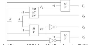
Fig. 11 Logical Diagram of QCA based 2:4 Decoder using CMVMIN Gate[5]
