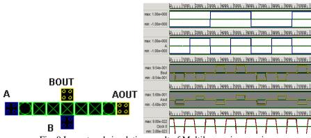
Fig. 9 Layout and simulation result of Multilayer wire crossing
