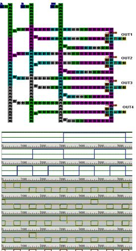
Fig. 16 QCA based 2:4 Decoder using 5 input Majority Voter Gate [9]
