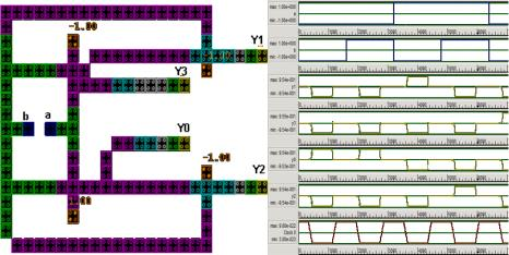
Fig. 12 Layout and Simulation of QCA based 2:4 Decoder using CMVMIN Gate
