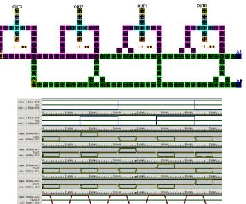
Fig. 14 Layout and Simulation result of QCA based 2:4 Decoder using Multilayer Wire Crossings [Traditional Method]
