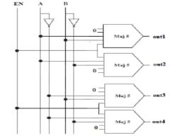
Fig. 15 QCA based 2:4 Decoder using 5 input Majority Voter Gate
