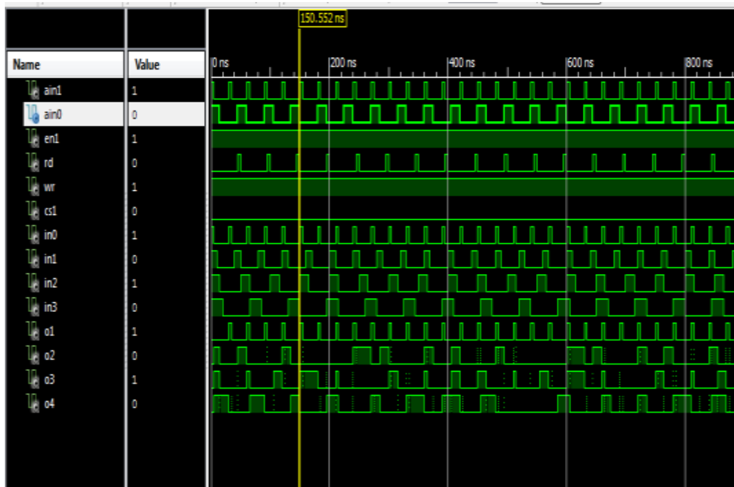
Fig.5 Simulation results for four bit memory.
