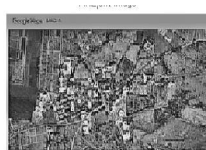
Figure 3.4 Adaptive Histogram equalization of Enhanced image of satellite image of Gprec college,kurnool.
