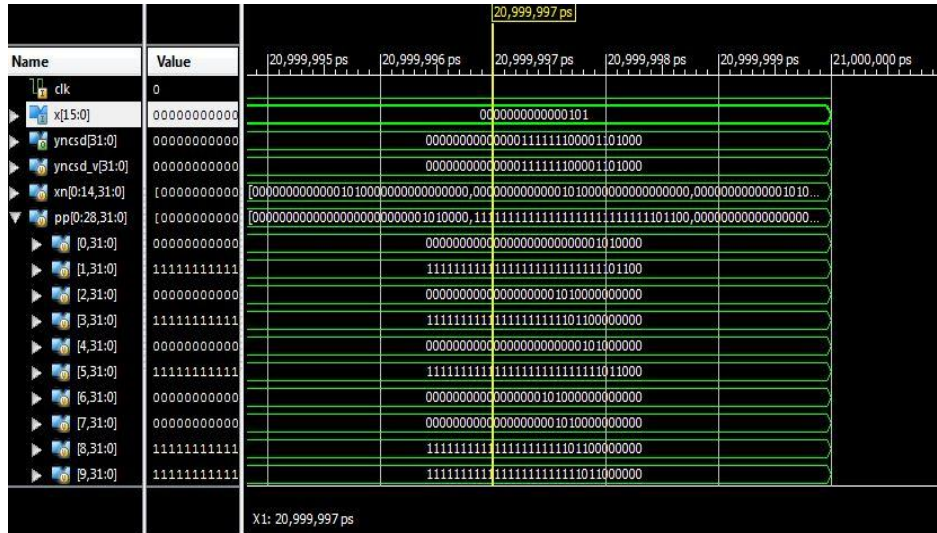
Figure 12. 15 tap FIR LPF output with CSD representation
