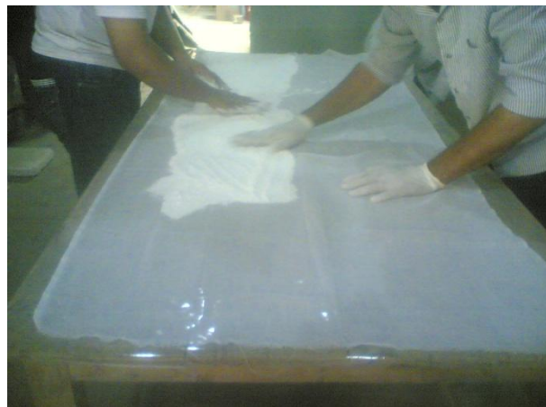
Figure (4) illustrates the process of spreading a layer of plaster and gauze on an external table
