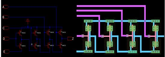
Fig.2 schematic and layout of 5-input AND gate (GDI tech)
