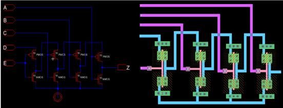
Fig.3 schematic and layout of 5-input OR gate (GDI tech)
