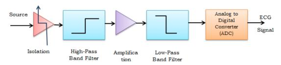
Fig.1: Architecture for acquisition of an ECG
