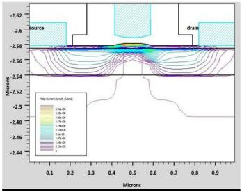
Fig.10 Total Current Density of Strained-Si pMOSFET
