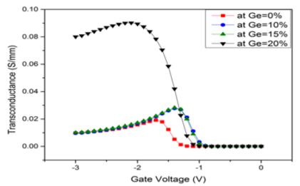
Fig.8 Transconductance at different Ge Concentration
