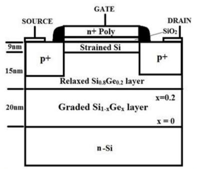
Fig.2 Cross Sectional View of Strained Si-pMOSFET
