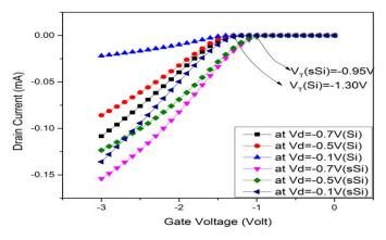
Fig.5 Current Drive Characteristic( $I_D \sim V_{GS}$ ) Curve
