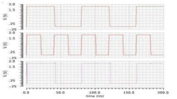
Figure 12: Simulation Design Implementation of SISO shift register
