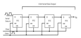
Figure 1: Circuit diagram of SISO shift register
