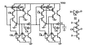
Figure 3: Master- Slave D flip flop circuit implemented using BICMOS
