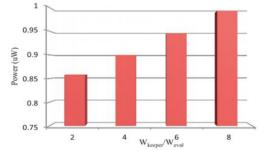
Fig.3 Effect of keeper sizing on power consumption of FLDL domino logic circuit
