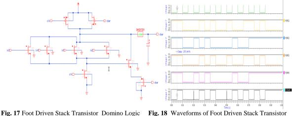
18 Waveforms of Foot Driven Stack Transistor Domino Logic
