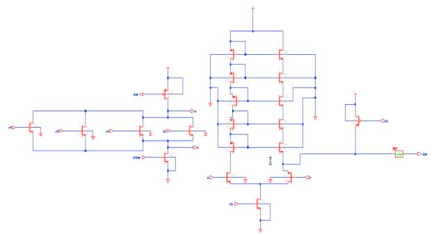
Fig 19. Comparator based domino logic for wide fan-in OR gate
