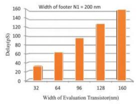
Fig.10 Effect of evaluation transistor width on delay
